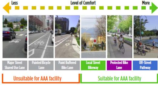
Continuum of Bikeway Facilities on Arterials without Curb & Gutter
